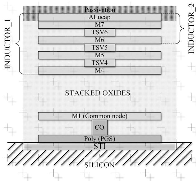
Fig. 3. Layer stack profile of the inductor based on CMOS 90 nm technology
