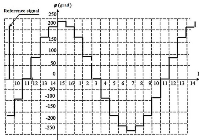
Fig. 3. Sample of the phase differences between the RV and CV of the AC while taking the bearings of an on-board radio station operating at a frequency of 125 MHz, with bearing of  $45^{\circ}$  and elevation angle of  $0^{\circ}$
