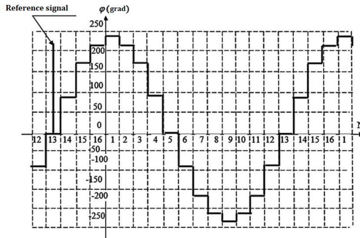
Fig. 2. Sample of phase differences between RV and CV of the AS while taking the bearings of an on-board radio station operating at a frequency of 125 MHz, with bearing of  $0^{\circ}$  and elevation angle of  $0^{\circ}$
