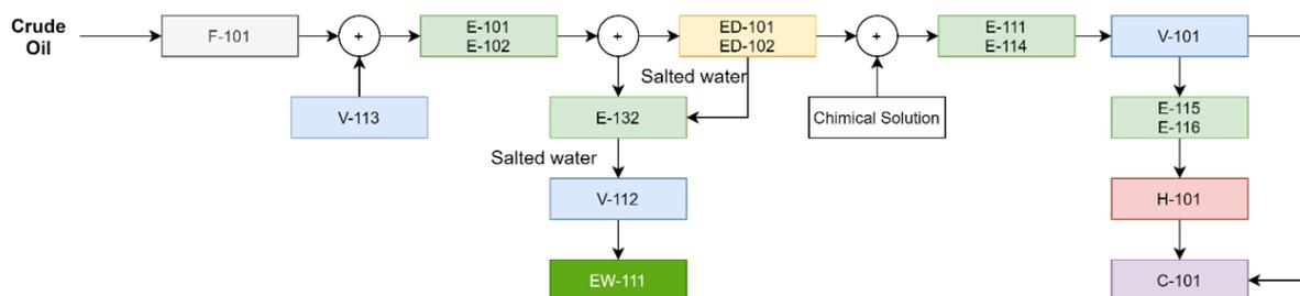
Fig. 2. Technological process of a desalination unit in oil manufacturing
