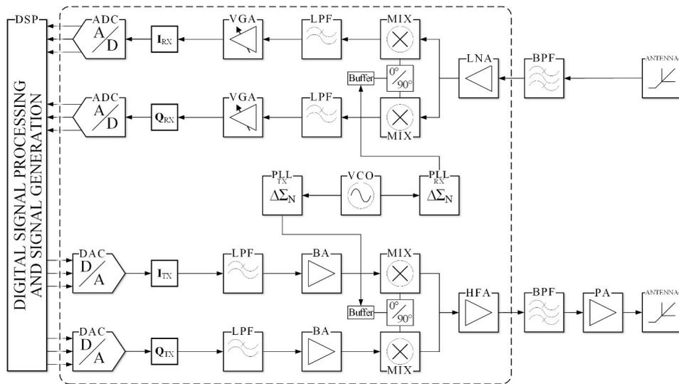
Fig. 1. Functional diagram of the NB-IoT transceiver
