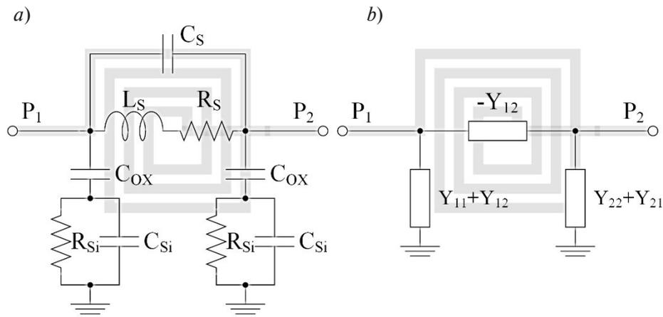
Fig. 2. IC inductor: *a* – lumped circuit; *b* – pi-model
