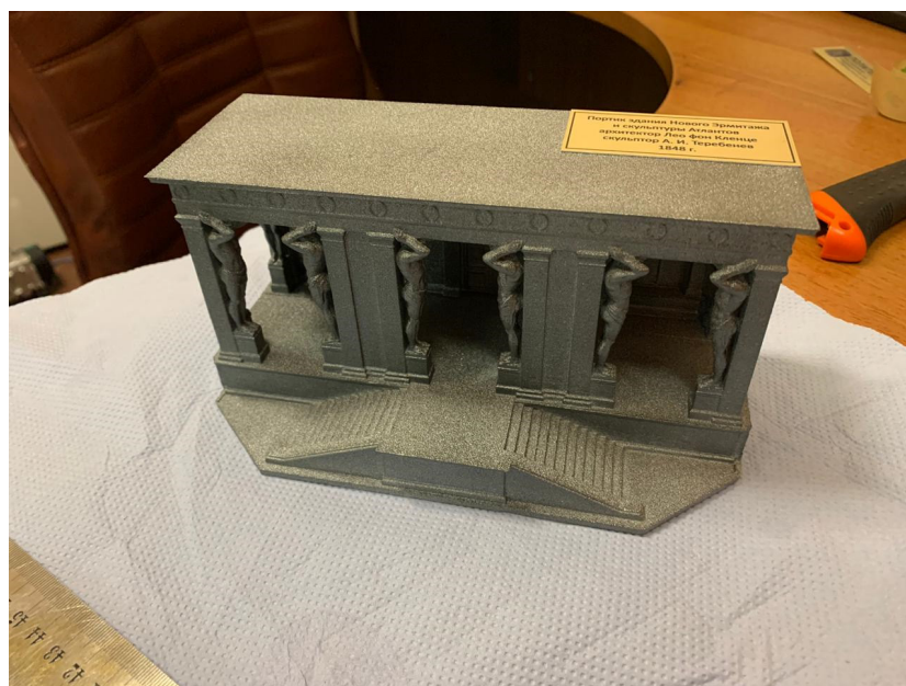
Fig. 5. A copy of the portico of the New Hermitage, printed on a 3D printer
