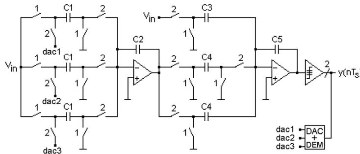
Fig. 1. Simplified structure of the unbalanced 2<sup>nd</sup> order delta-sigma modulator
