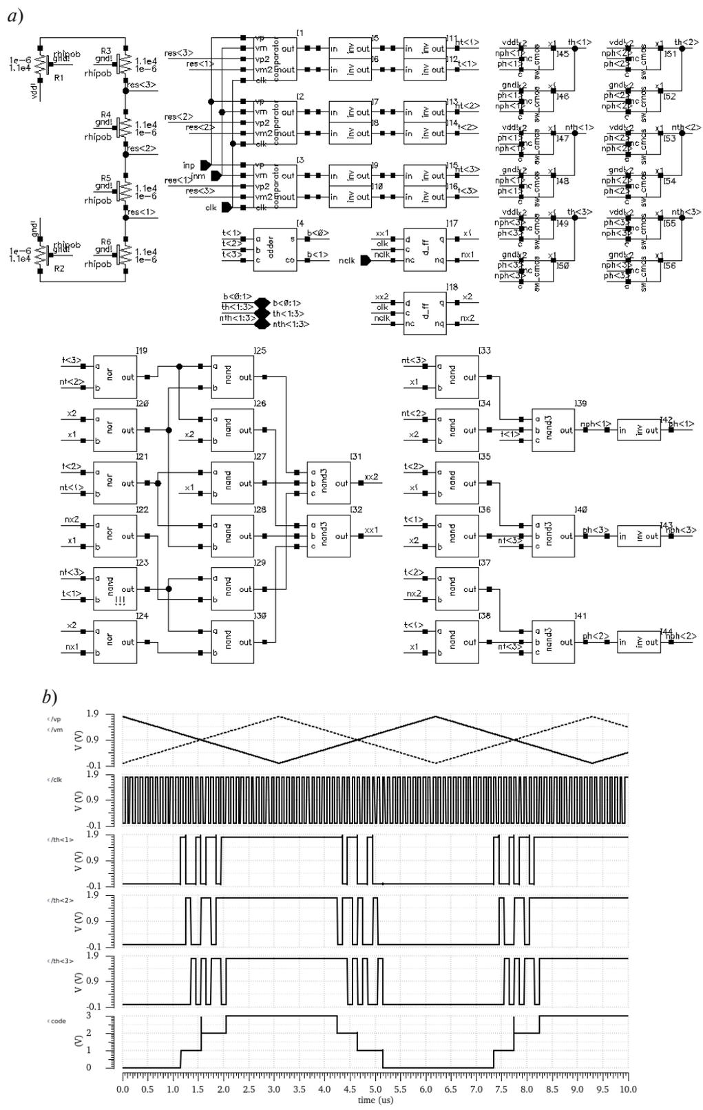
Fig. 4. Circuit of ADC-DAC part with DEM (a); Simulation results (b)
