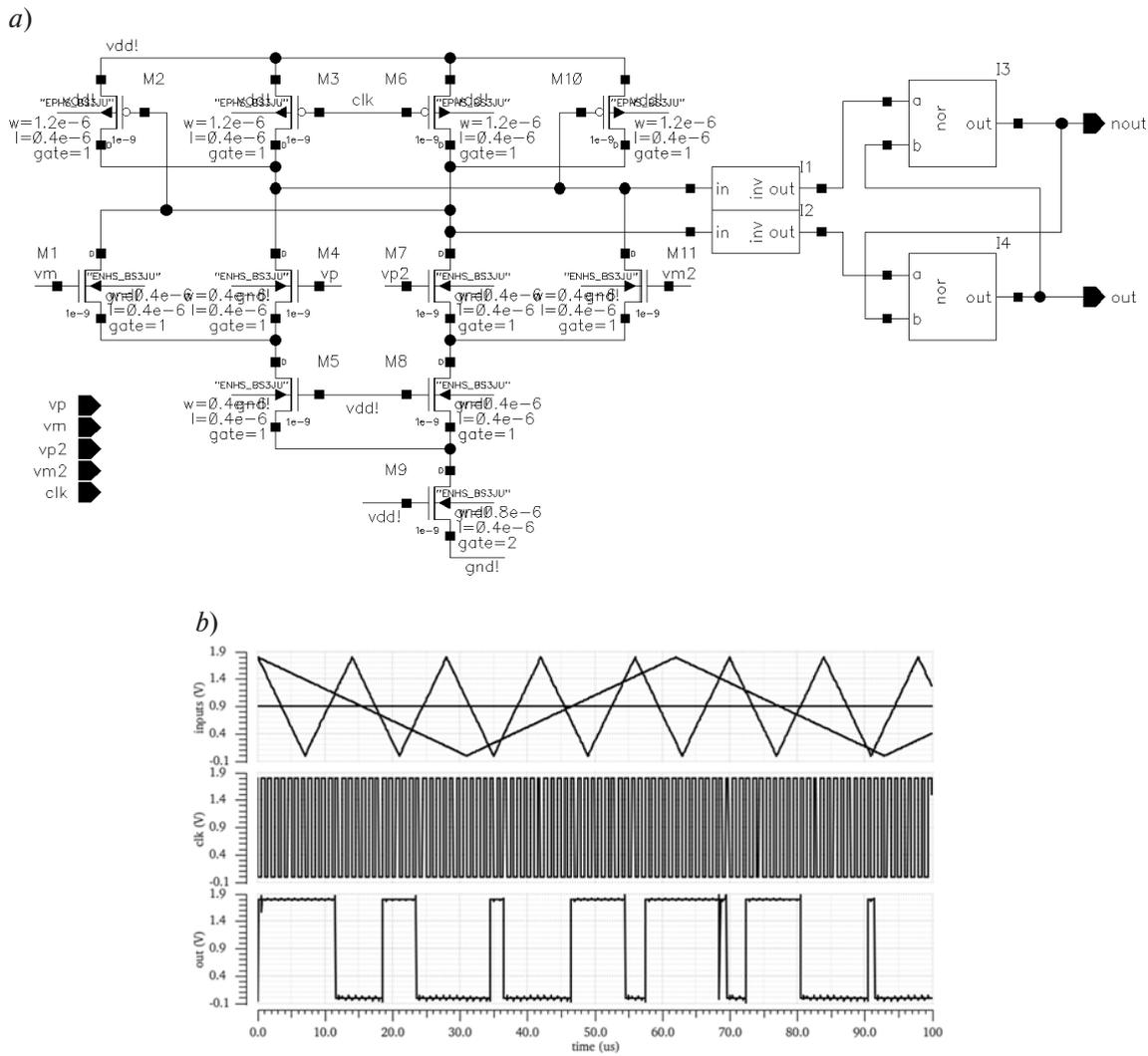
Fig. 3. Circuit of differential comparator (a); Simulation results (b)
