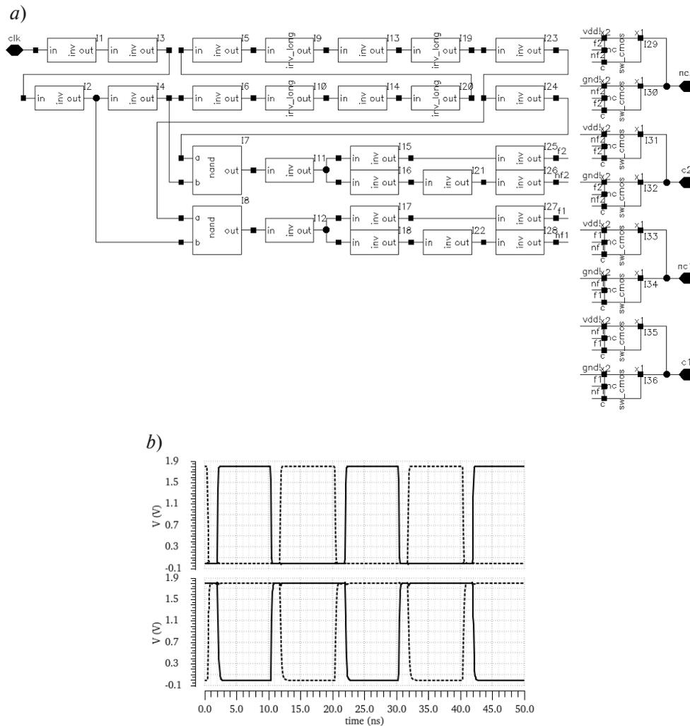
Fig. 2. Circuit for generating signals of the first and second phases (a); Simulation results (b)
