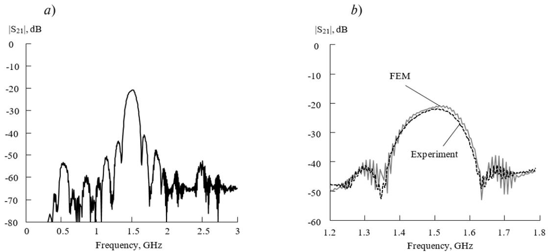
Fig. 6. Frequency response: *a* – calculated without “parasitic” LC-elements; *b* – calculated with “parasitic” LC-elements and experimental
