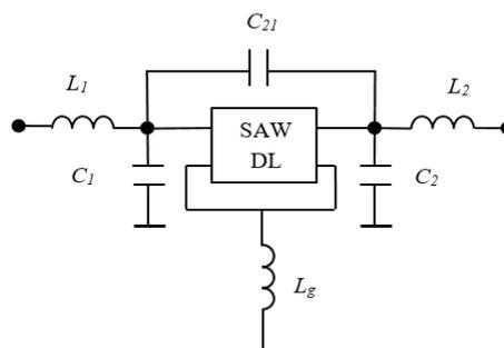
Fig. 7. Scheme with “parasitic” LC elements
