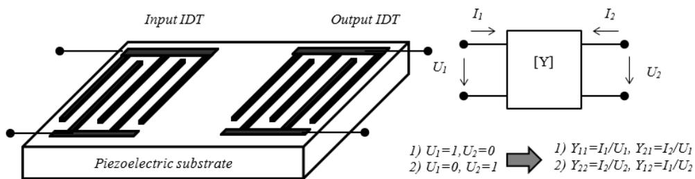
Fig. 1. SAW delay line: a – typical topology; b – the device in the system of Y-parameters and the principle of switching electrical ports for finding Y-parameters
