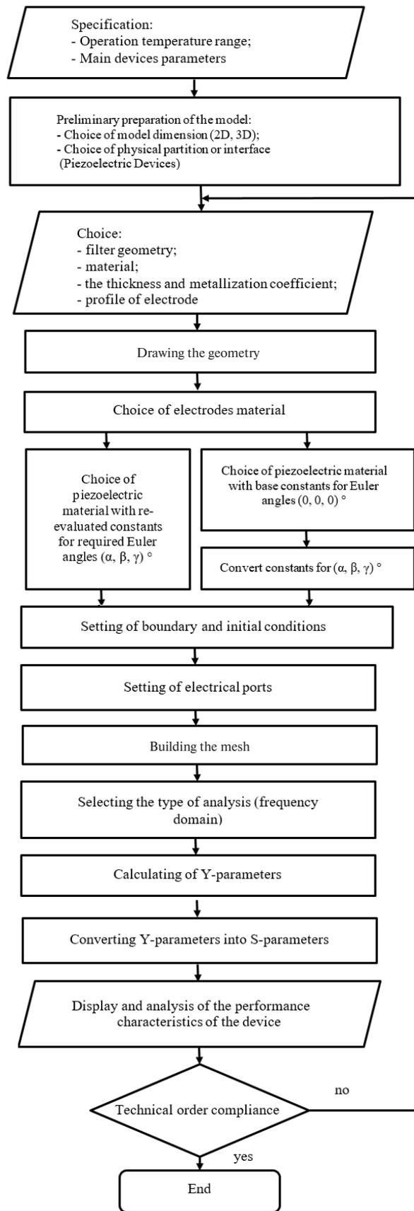
Fig. 4. Calculation algorithm in COMSOL
