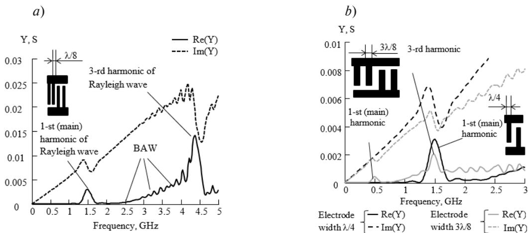
Fig. 3. Principle of operation of the IDT at harmonics: *a* – fundamental and 3<sup>rd</sup> harmonic of the IDT with split electrodes (width of electrodes  $\lambda/8$ ); *b* – fundamental and 3<sup>rd</sup> harmonic excitation for IDT with split electrodes (electrode width  $3\lambda/8$ ) and only fundamental for IDT with  $\lambda/4$  electrodes
