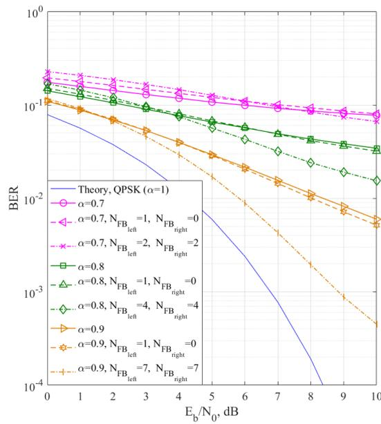
Fig. 8. Comparison of standard demodulation algorithm, asymmetrical feedback algorithm on one subcarrier ( $N_{FB\_left} = 1$ ) and symmetrical feedback algorithm
