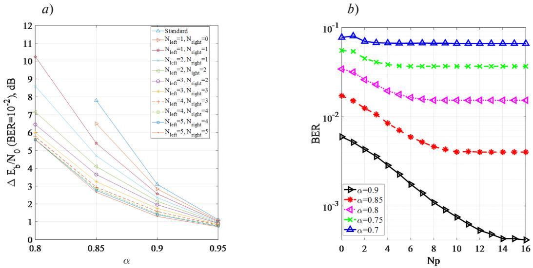
Fig. 7. a – Dependence of energy loss versus  $\alpha$  at various  $N_{FB}$  ( $BER = 10^{-2}$ );
