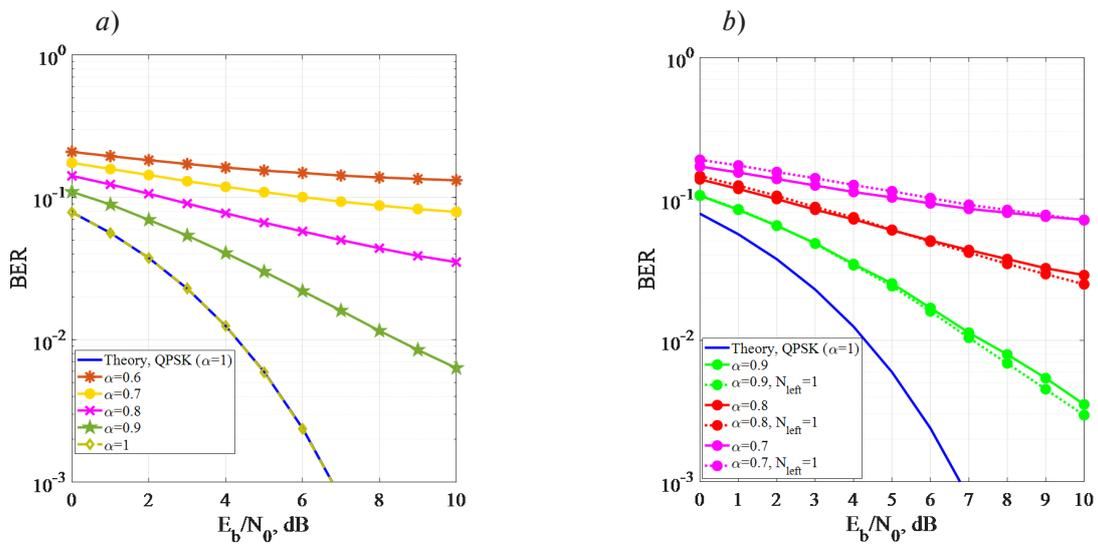
Fig. 6. BER performance: a – SEFDM signal with various  $\alpha$  ( $N = 256$ ); b – comparison of standard demodulation algorithm and asymmetrical FB demodulation algorithm ( $N = 32$ ,  $N_{FB\_left} = 1$ )
