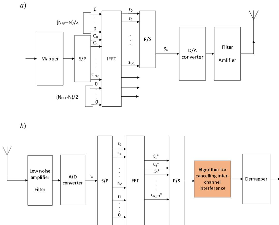
Fig. 1. Structure scheme of transmitter and receiver
