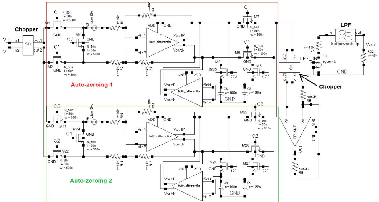
Fig. 7. Schematic of an amplifier using both chopping and auto-zeroing
