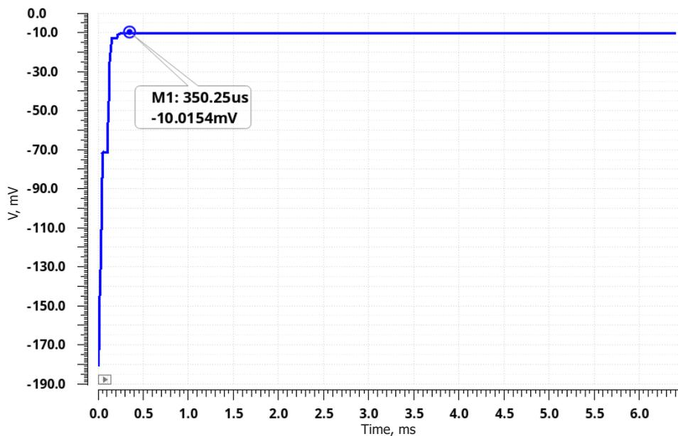
Fig. 2. Voltage on capacitor C0 versus time
