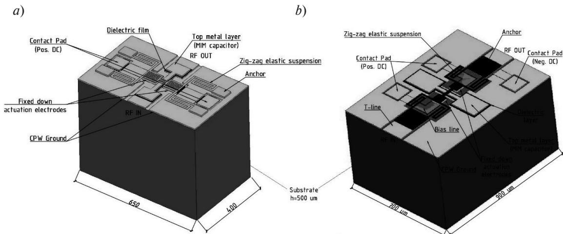
Fig. 1. 3D topology of the RF MEMS switch: *a* – 1<sup>st</sup> type; *b* – 2<sup>nd</sup> type
