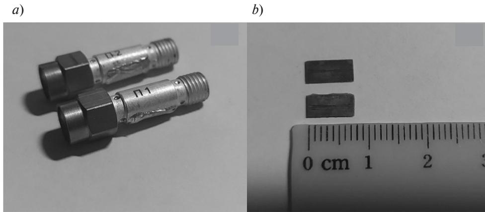
Fig. 2. Manufactured experimental samples of RF MEMS switches:
