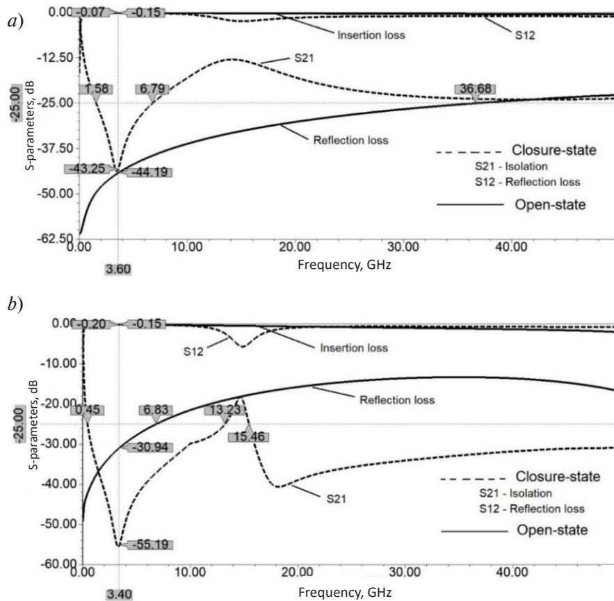
Fig. 3. Results of measuring the electromagnetic parameters experimental samples of RF MEMS switches: *a* – 1<sup>st</sup> type; *b* – 2<sup>nd</sup> type
