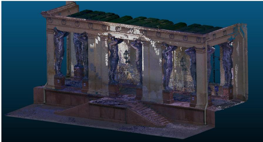
Fig. 2. The resulting point cloud
