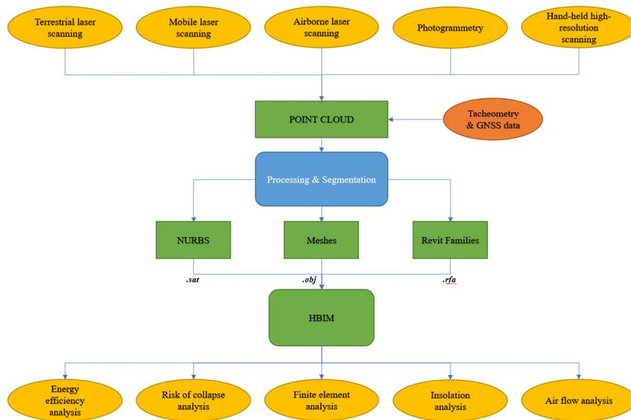
Fig. 1. Block diagram of the developed technique
