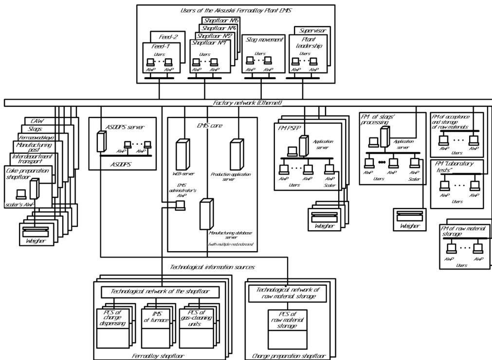
Fig. 2. Structure of EMIS of the Aksuskkii Ferroalloy Plant:
