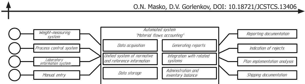
Fig. 1. Functional structure of the automated system "Accounting of material flows" of the metallurgical shopfloor of the Copper Plant
