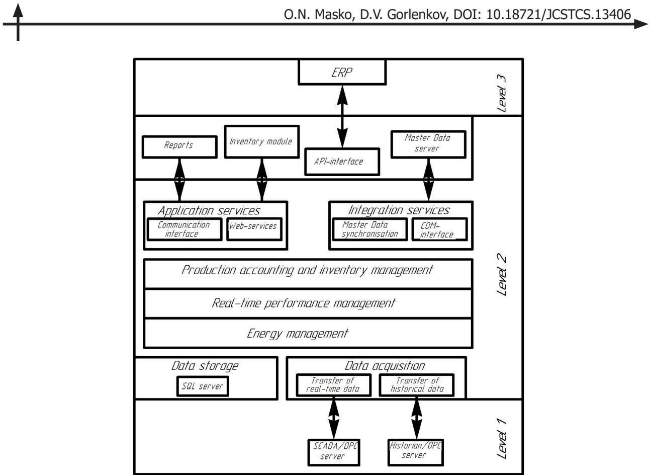
Fig. 3. The generalized structure of the project of the automated material flow management system,
