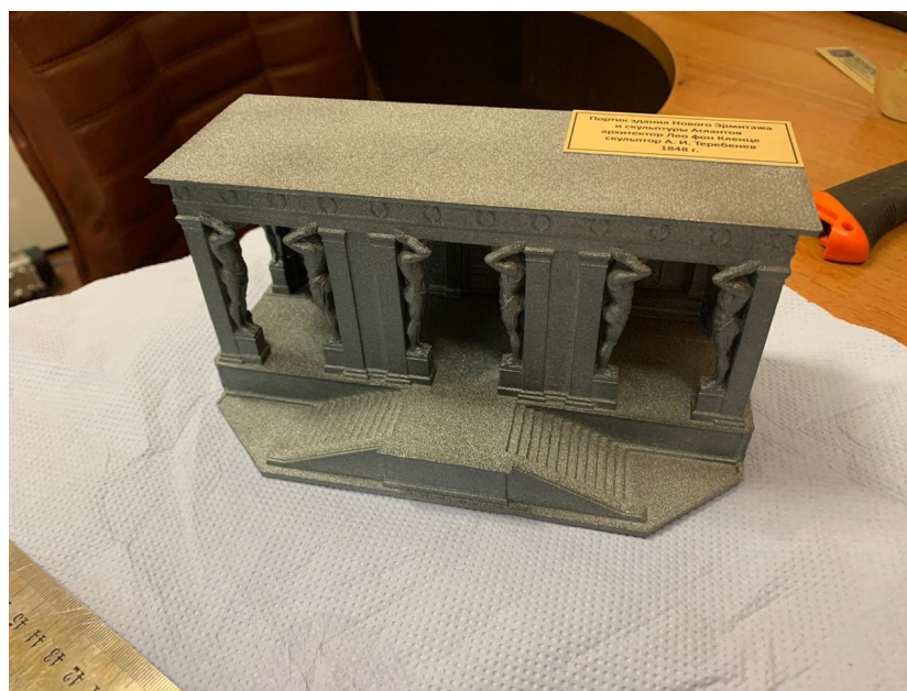
Fig. 5. A copy of the portico of the New Hermitage, printed on a 3D printer
