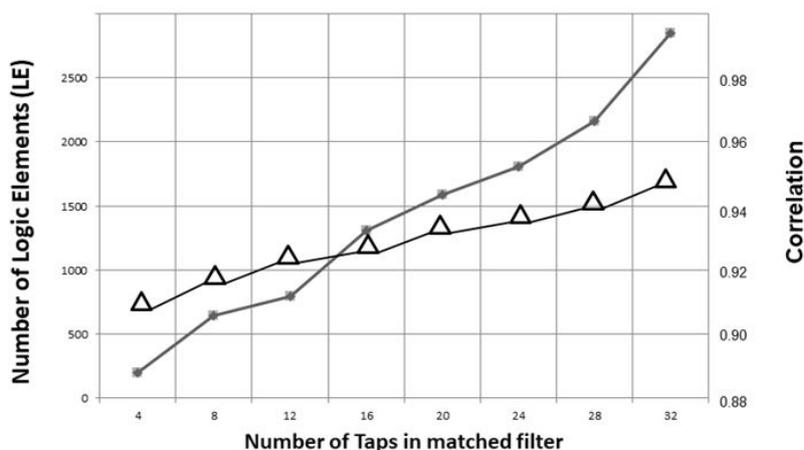
Fig. 2. Correlation values and number of logic elements (LE) depending on the number of taps in the correlator
