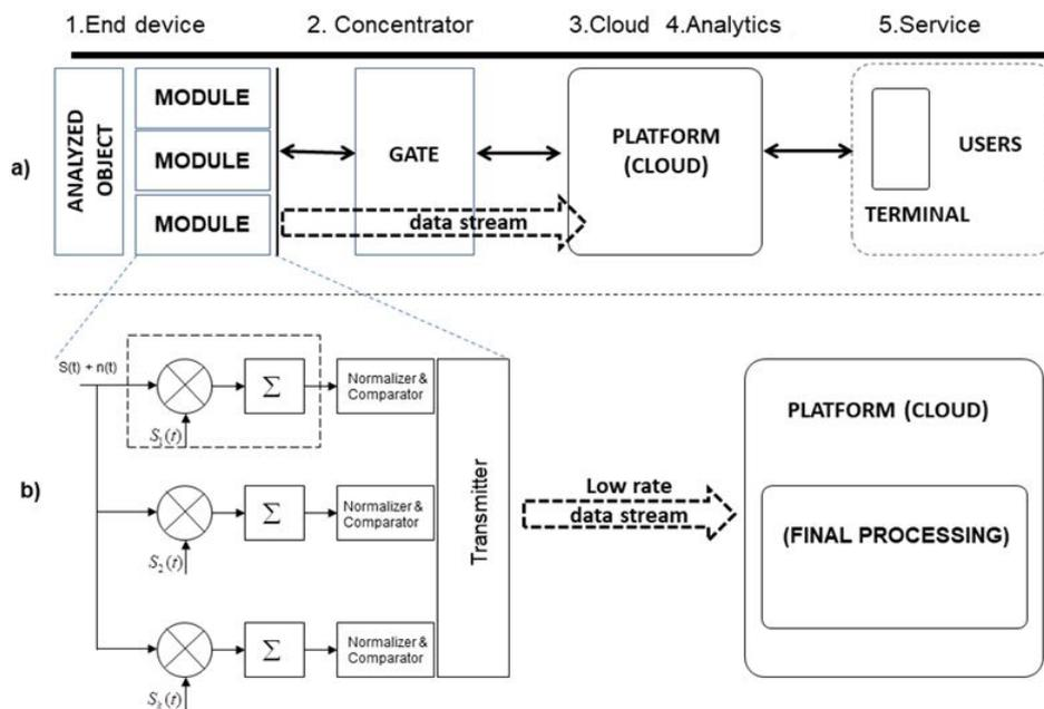
Fig. 1. Typical architecture of IoT systems (a) and simplified block diagram for a matched filter in a module and low rate data transmission to a cloud (b)
