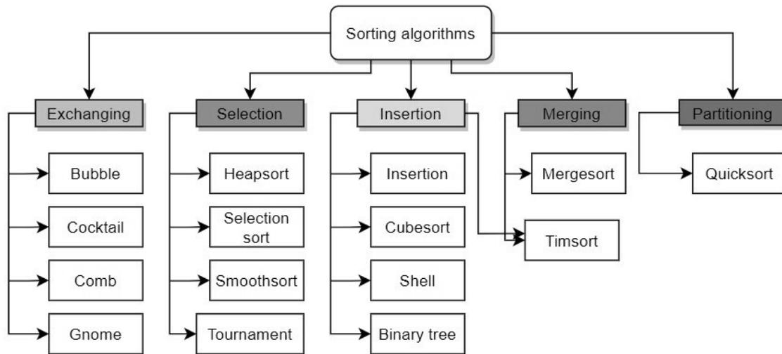
Fig. 1. A simplified classification of sorting algorithms
