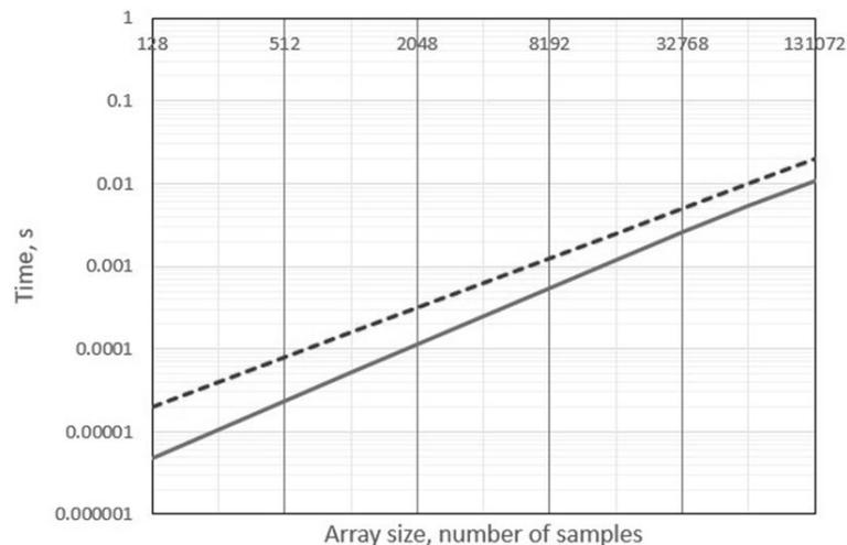
Fig. 5. Dependence of merge sorting time on array size
